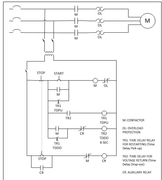
Fig. 1 Simplified motor restarting using electromechanical time relays
