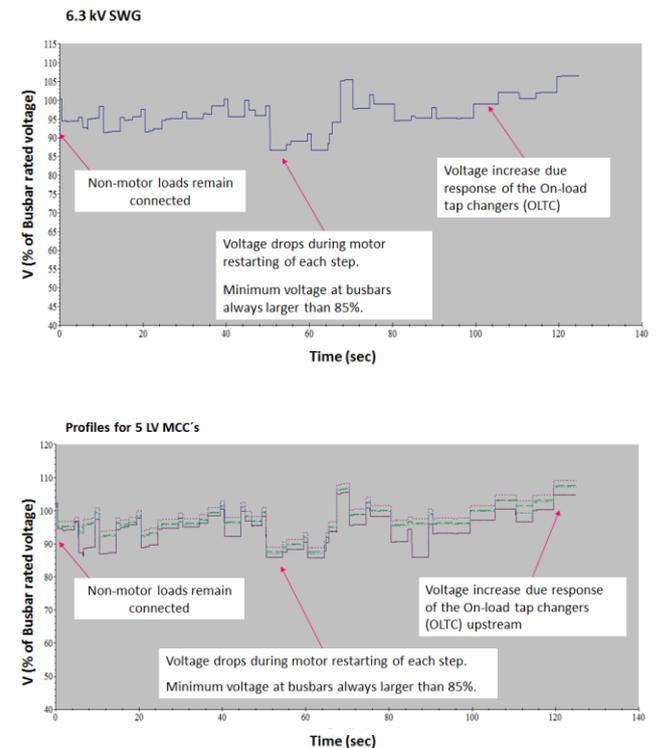
Fig. 6 Typical voltage profile in MV and LV switchgears during restarting of MV and LV motors
