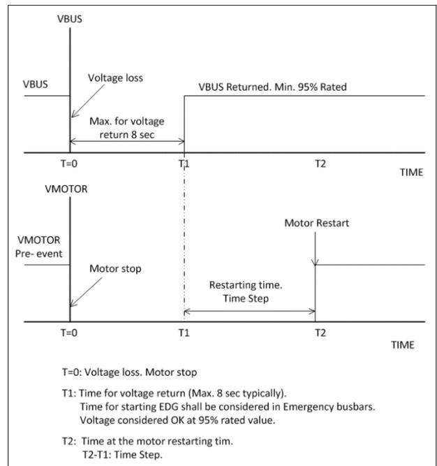
Fig. 3 Total time involved in a motor automatic restarting
