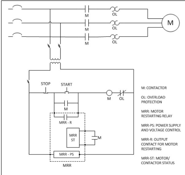
Fig. 2 Simplified scheme using a dedicated electronic restarting relay.
